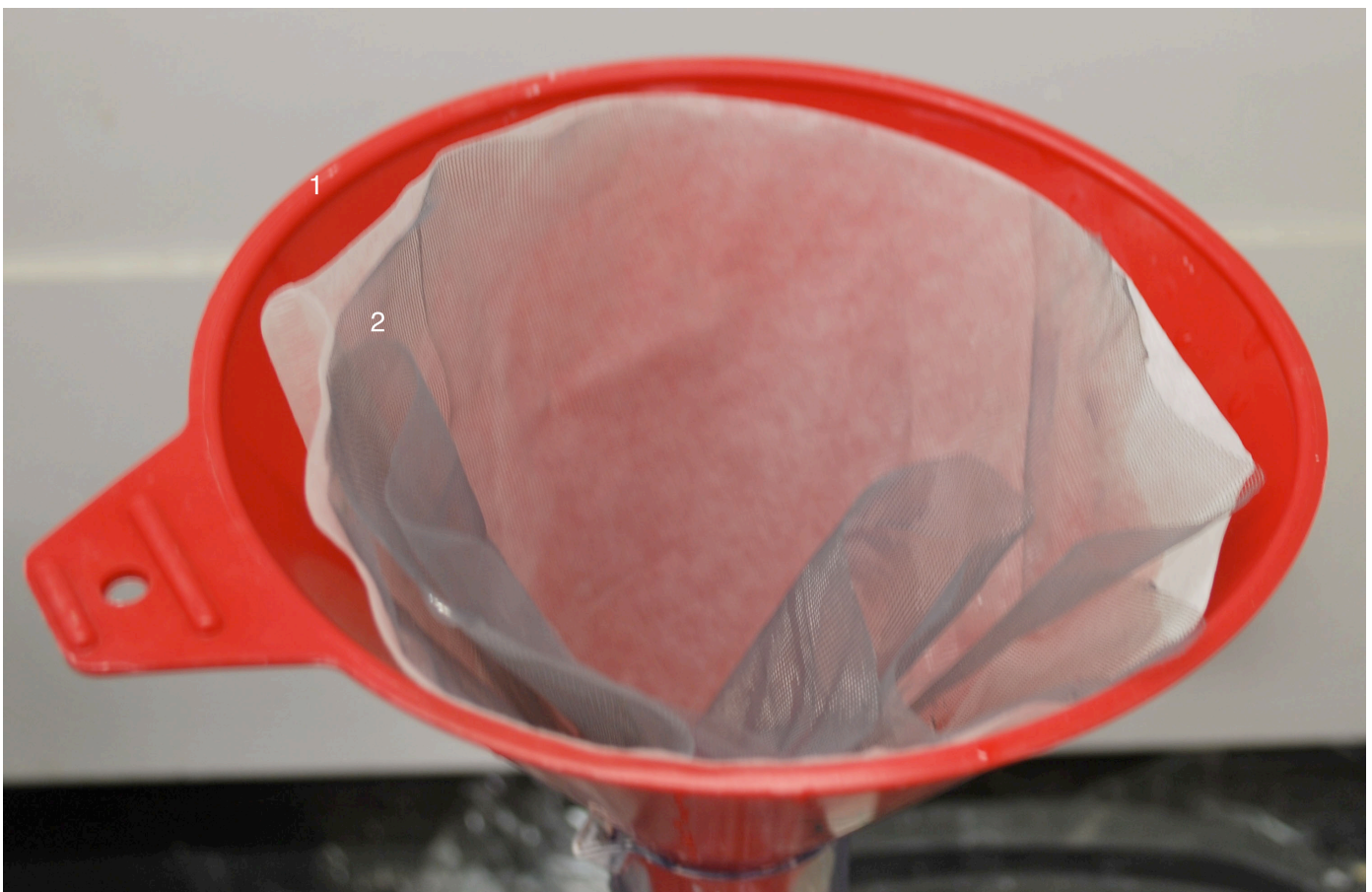
Figure 3. A close-up of the funnel apparatus with the outer plastic funnel (1) and inner mesh net (2).
